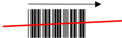
Fig. 14. A picket code and scan line angled to 'see' more of the code height
