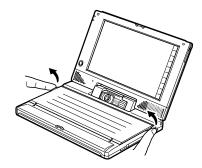
**NOTE:** Keep the keyboard hard cover, it is reusable. Replace the cover the same way you removed it.
