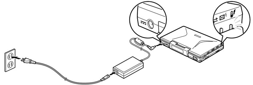
11. When charging is completed, disconnect the AC adapter and the power cord.
