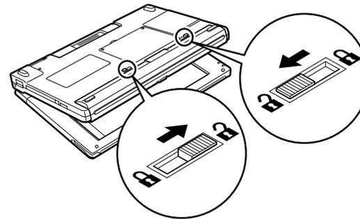
3. Align the main battery pack with the rails of the 6651 and push it straight in.
