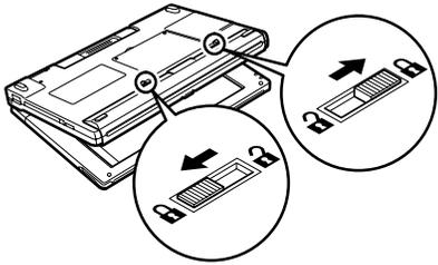
► **NOTE:** Both lock switches must be locked or the 6651 won't power on.
