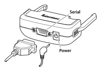
You must remove the serial adapter from the CK60 to insert the handheld computer into a dock.
