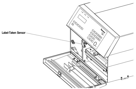
The photoelectric sensor emits a narrow beam of light, which will be reflected back to the sensor by any label, ticket, tag, piece of strip or backing paper, that has not been removed from the outfeed area. A prerequisite is that the web is fed out along the inner wall of the printer.
