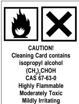
We recommend using the special *Cleaning Card* (part number 1-110071-00) and the procedures below to clean the printhead before loading each new roll of labels or tags.
