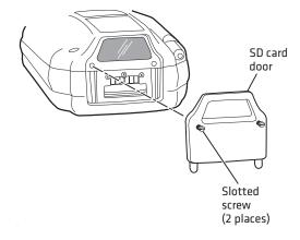
**6** Insert the SD card that contains the upgrade files into the CK31G. Make sure that the contact pins are facing up and that the SD card clicks into place when you insert it.
