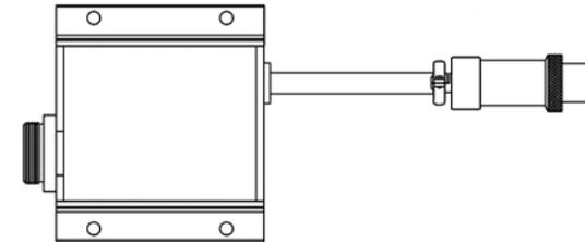
The dongle cable (P/N 851-070-101) is a device that prevents damage to the DC/DC converter (P/N 851-070-001) caused by frequent battery connection/disconnection on electric forklifts.
