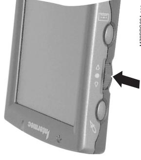
2. Pull the stylus out of its built-in compartment.
