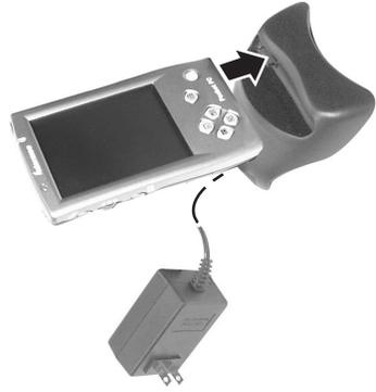
6. Dock the Pocket PC in its cradle and charge for at least 3 hours. You can use the Pocket PC while the battery is charging.
