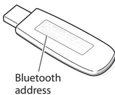
**Bluetooth Adapter Bluetooth Address:** The Bluetooth adapter Bluetooth address is located on the bottom of the label on the adapter.
