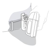
When you let go of the CK1, the weight of the computer makes it swing down so that it hangs vertically with the screen at the top.
