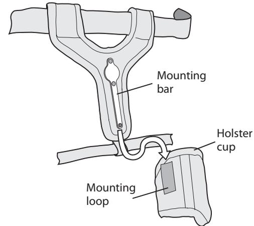
3 The holster cup has two more mounting loops in addition to the one that you slid off of the mounting bar in Step 2.
