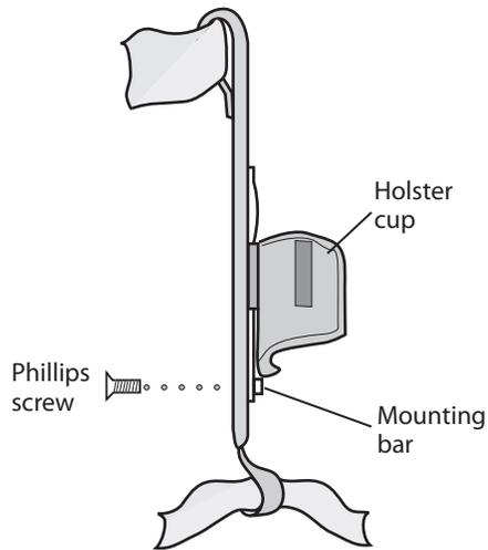
2 Slide the holster cup down and off of the mounting bar.
