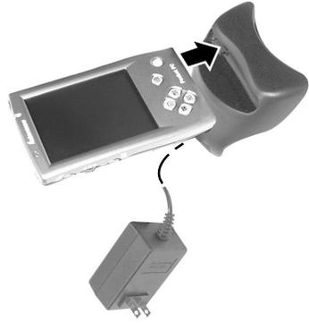
6. Dock the Model 70 in its cradle and charge for at least 30 minutes. You can use the Model 70 while the battery is charging.
