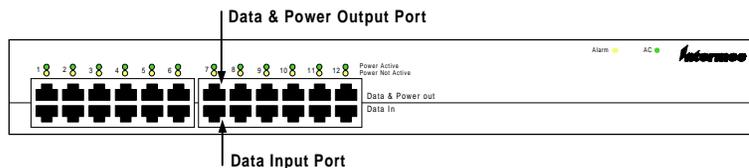
**10BaseT/100BaseTx Data Input Ports, Lower 6/12 Ports** The Power Bridge has 6/12 10BaseT/100BaseTx data input ports, configured as Media Dependant Interface (MDI) (non-crossover). These ports are designed to carry Ethernet data only (Tx/Rx) over the standard 2-wire pairs (RJ-45 pins 1/2 and 3/6).
