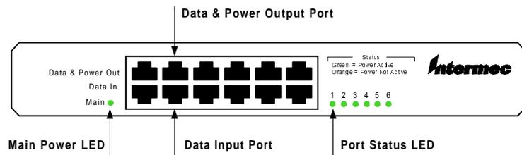
The next illustration shows the LEDs and ports of the 12-port Power Bridge. The LEDs and ports are explained in the next sections.
