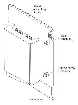
For additional security, you can supply a padlock and insert it through the bracket and bracket support.
