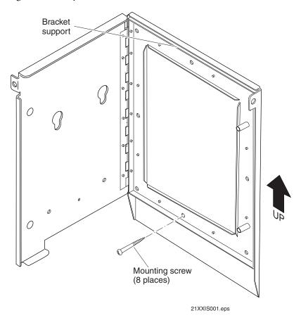
**5** If needed, use additional hardware to secure the bracket to the mounting surface.
