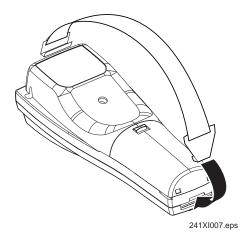
You will need to release the handstrap to remove and install the battery pack.
