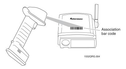
After a 3 to 4 second pause, the scanner will beep once and the green light on the base will flash. If the scanner beeps three times after 3 to 4 seconds, the scanner did not associate to the base. Make sure that there are no more than nine scanners associated to the base.
