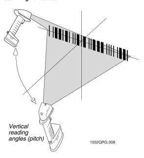
2. If you did not get a good read, adjust the scanner distance from the bar code and the position of the scan beam to make sure you scan every bar and space.
