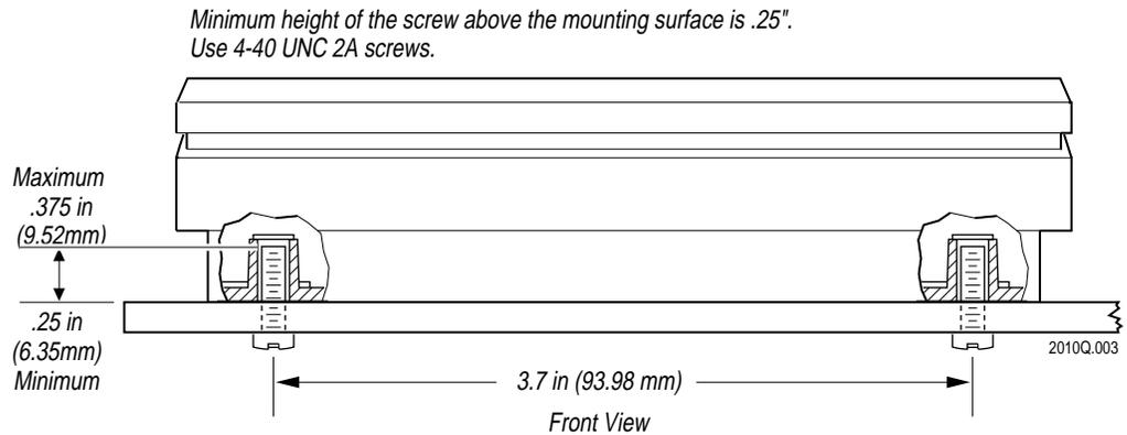
**Note:** If you mount the JZ2010 battery charger on a table top or shelf, make sure you have enough vertical clearance to insert and remove battery packs easily. Also remember to leave space behind the charger so that you can connect the power supply and reach the discharge button on the back panel.
