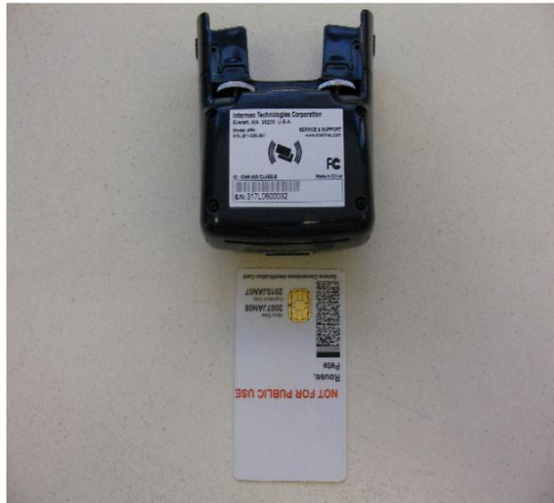
**Figure 1 – How to insert a SmartCard into the PIV**
